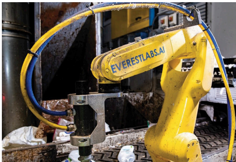
Above: Everest Labs’ RecycleOS platform combines AI with robotic sorting
